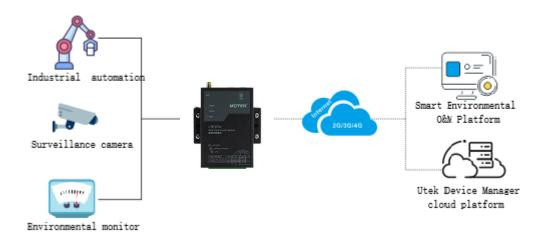
D9701 series DTU products are especially suitable for the application of data collection and monitoring of distributed unattended sites, and remote configuration and management through the equipment management cloud platform.
