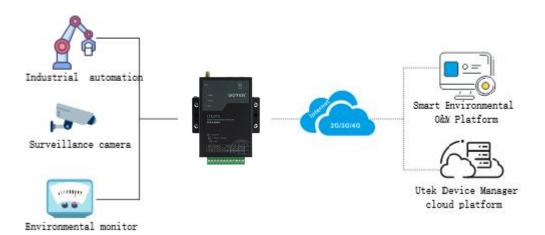
D9201 series DTU products are especially suitable for the application of data collection and monitoring of distributed unattended sites, and remote configuration and management through the equipment management cloud platform.
