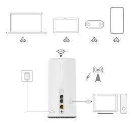
2. Access the Internet via Ethernet (through an ONT or other WAN-connected device).
