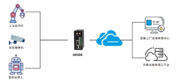
G9306 series 4G industrial gateway, supporting 4G/3G/2G, WiFi, wired network and other access methods, can realize local real-time data pre-processing, data analysis. And
