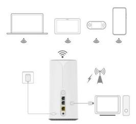
2. Access the Internet via Ethernet (through an ONT or other WAN-connected device).
