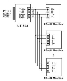
3. Half-duplex communication connections between UT-503 interfaces
