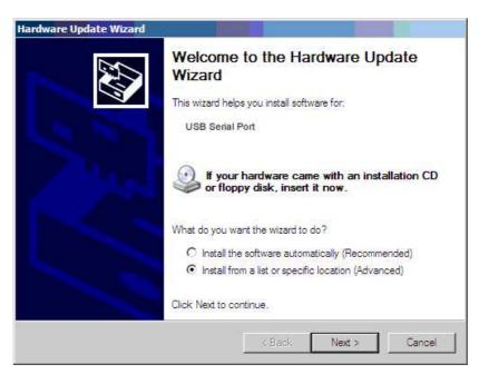
The system has found the hardware installation information of the USB Serial Port as shown in the figure below, then click "Next".
